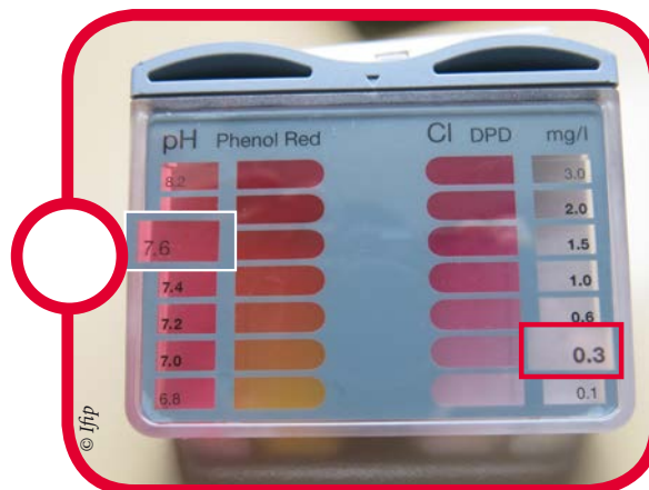
Concentration en chlore insuffisante
